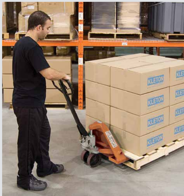
3-function hand control (raise, neutral and lower) and spring-loaded self-righting safety loop handle.
